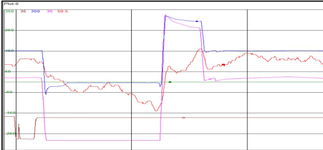
Fig. 5. Operational Transition from Generate Spin to Generate (reaching 300MW in less than 10 seconds) triggered by significant LF event. Notice the correction of grid frequency thanks to this large pumped storage unit.
