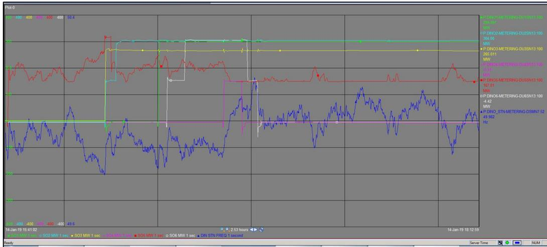
Fig. 8. All Six Dinorwig Units Respond to a Grid Emergency, adding 1,466 MW in minutes
