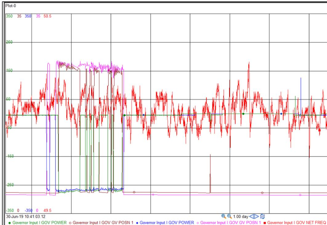
Fig. 7. Frequent Daytime Switching between Pump mode and Spin Pump mode
