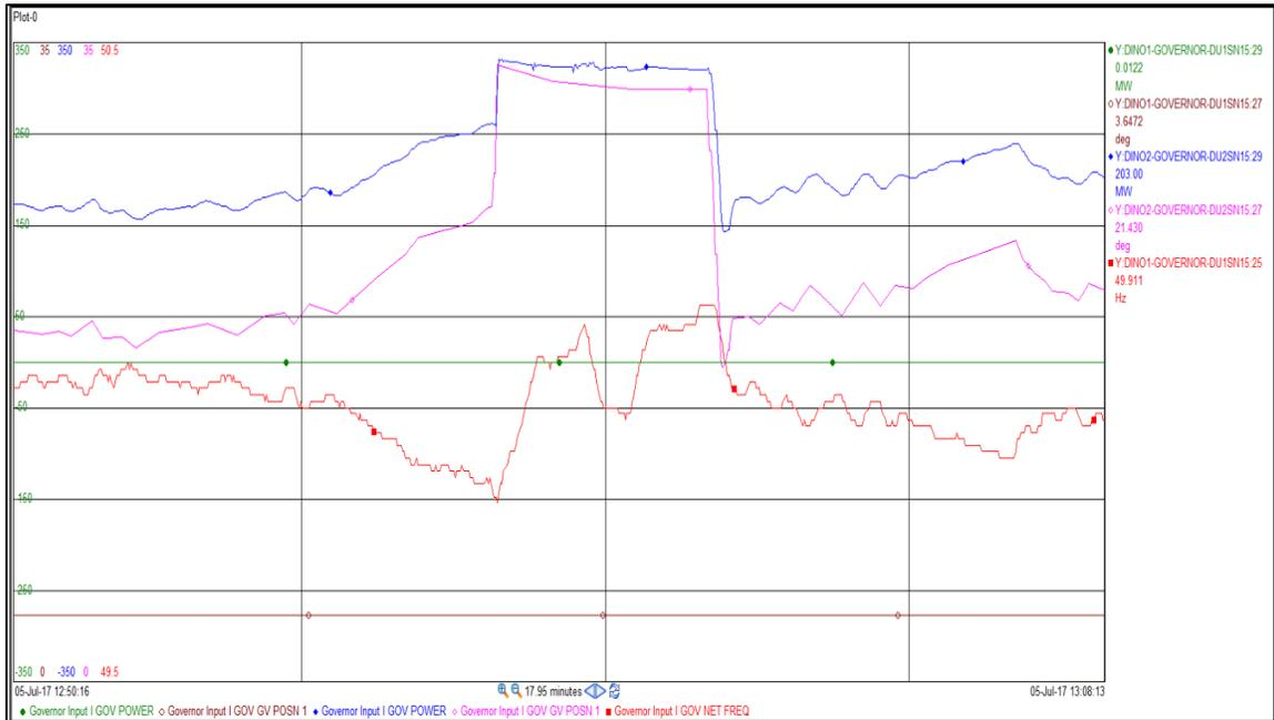
Fig. 4. Typical LF response during Generate mode. Governor software modifications in 2013 enabled Primary Frequency Response also when operating in Pump mode.
