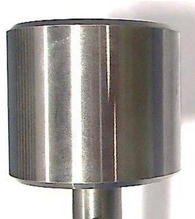
The dashpot is essentially a tunable shock absorber for the governor. If the dashpot plunger is scored or pitted from water or dirt, the reset time will diminish taking the governor longer to sync and losing stability. Only dashpot oil should be used in the dashpot and to oil linkages in order to avoid accidental contamination.
