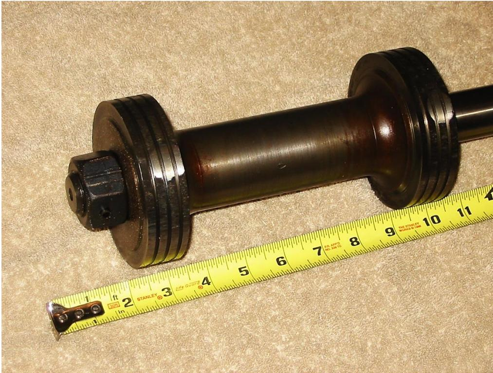
This distributing valve came from a MOD II Governor that had a series of unfortunate events occur. In this unit, the piston rings in the main servo motor came apart contaminating the oil with metal shavings. This in turn caused gouges in the piston, allowing oil to bypass and leak. The pumps began cycling continuously causing the oil to overheat and eventually caused the servos to go bad. The servos then needed to be bored out and replaced.
