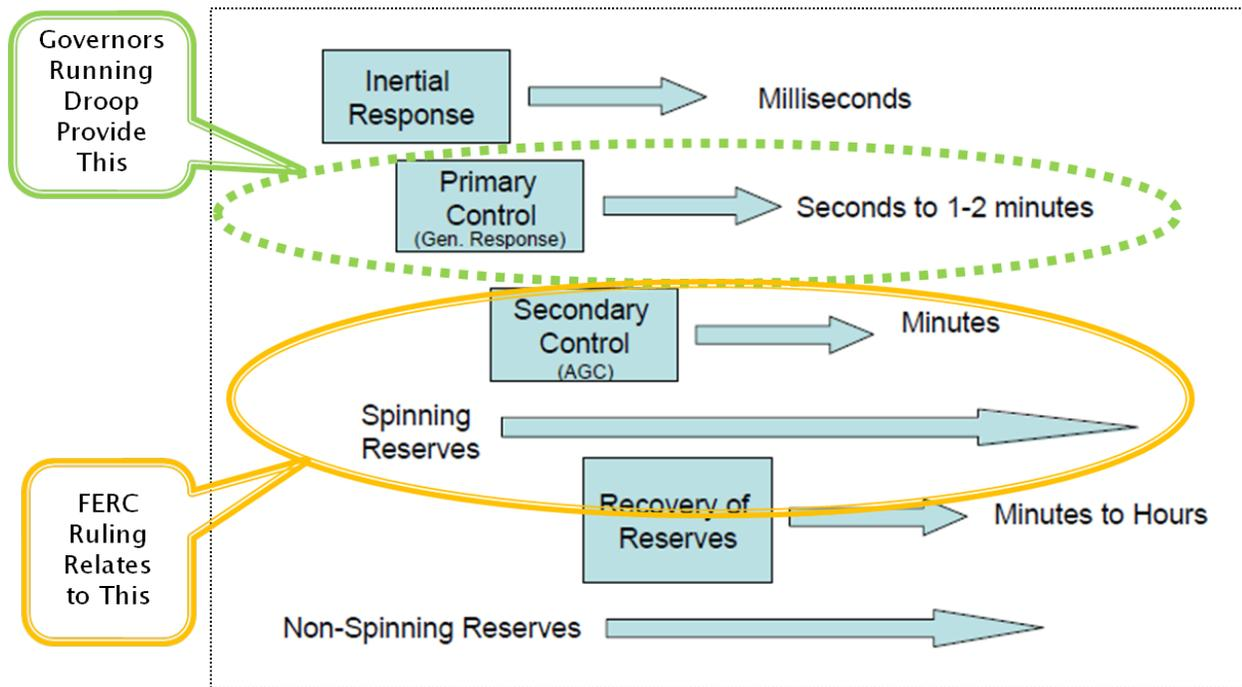
In short: the FERC ruling says that if individual generators are demonstrably and actively helping stabilize grid frequency, they should be rewarded financially. Conversely, if individual generators *cannot* or *do not* (due either to their current method of operation, pollution constraints, thermodynamic constraints, or other issues) actively respond to grid frequency excursions, they should only be paid for the real power generated *and nothing more*.
