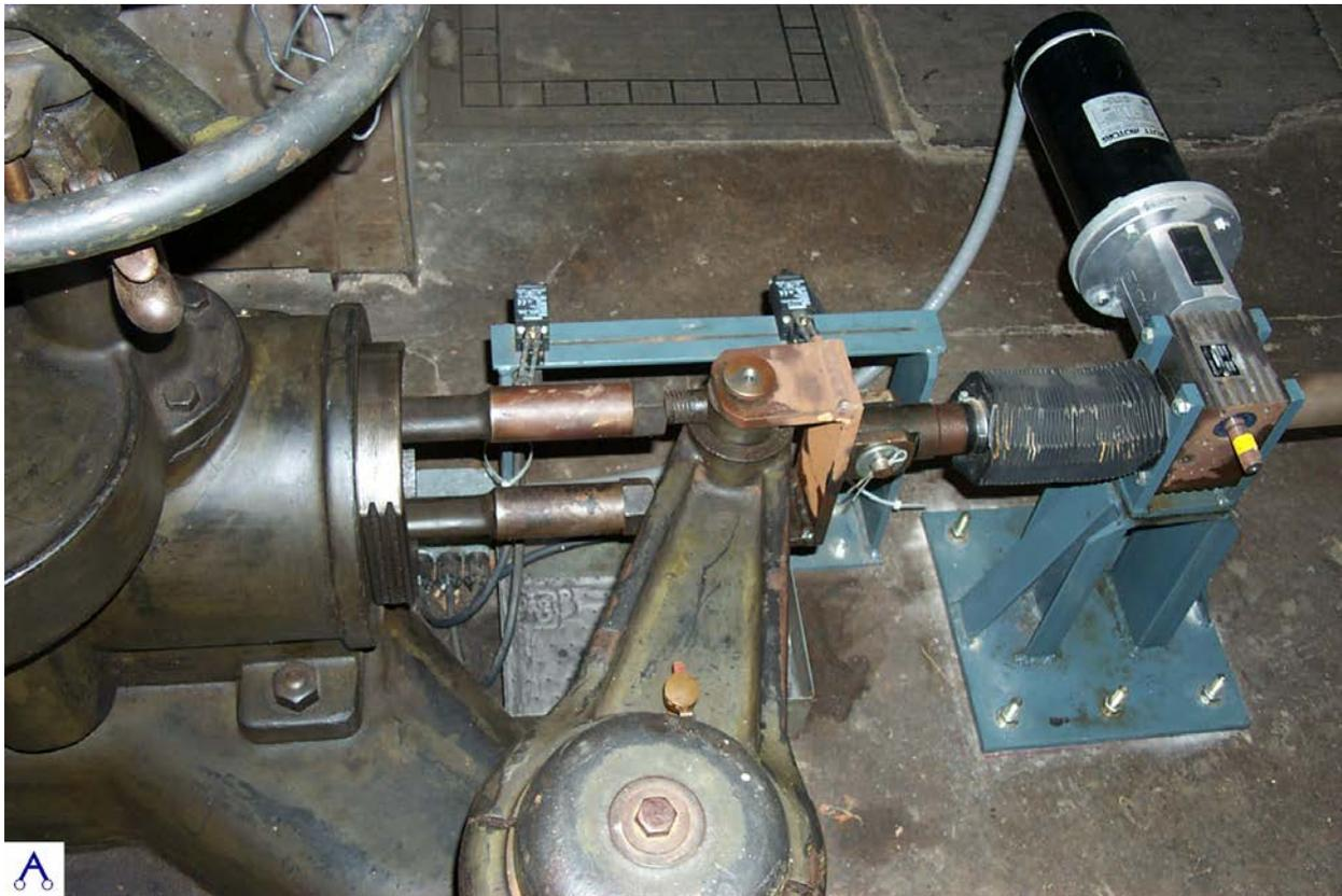
*The original Woodward Gateshaft governors were physically retained, but were converted with electrically operated rack & pinion gate position assemblies.*
