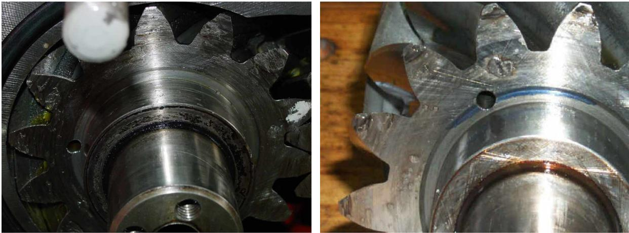
*Figure 3 - Pump Gear Damage*
