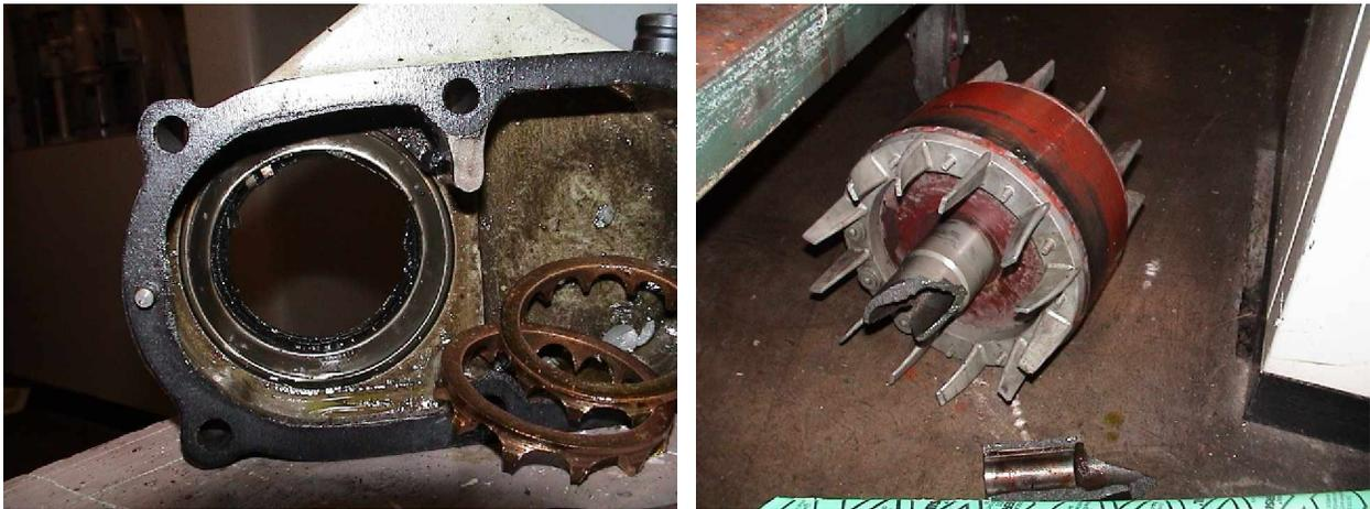
*Figure 6 - this pump stopped, the rotor didn't*
