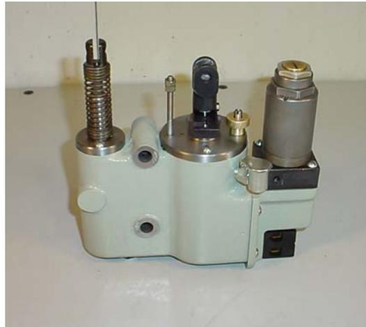
Figure 1 Dashpot with Solenoid Bypass
