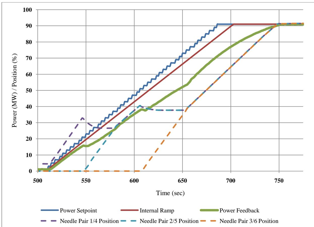
Figure 12 - Needle Sequencing at Stanislaus - Load On Ramp
