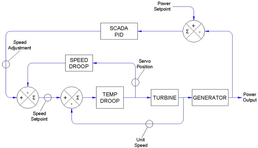
**Figure 8 - Simplified Block Diagram of Load Control with SCADA PID Controller of a Mechanical Governor**
