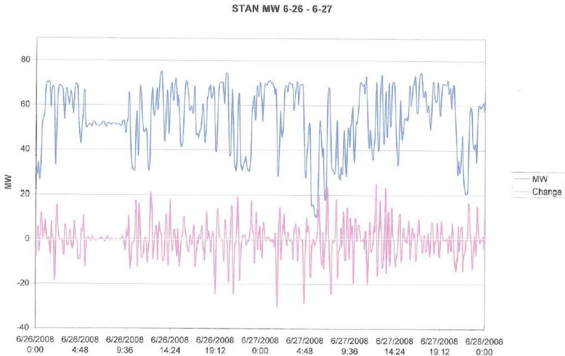
**Figure 4 – Typical Output of Stanislaus Powerhouse - Two Day Period**
