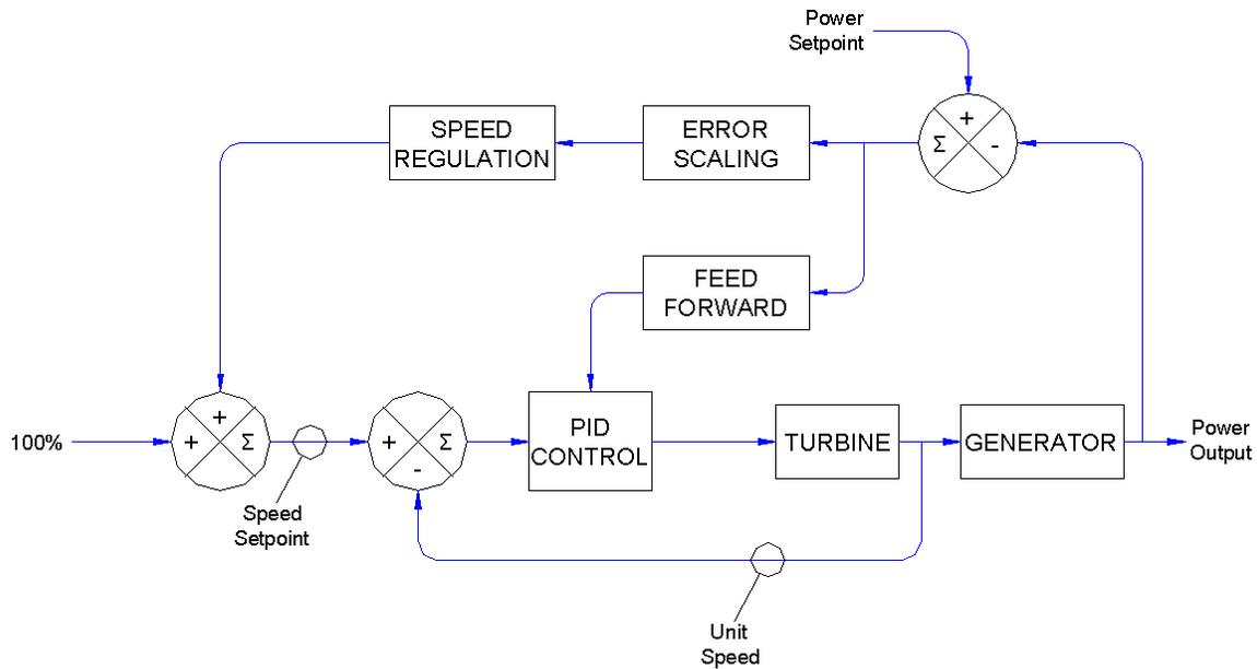
Figure 10 - Simplified Block Diagram of Load Control with Speed Regulation and PID Digital Governor
