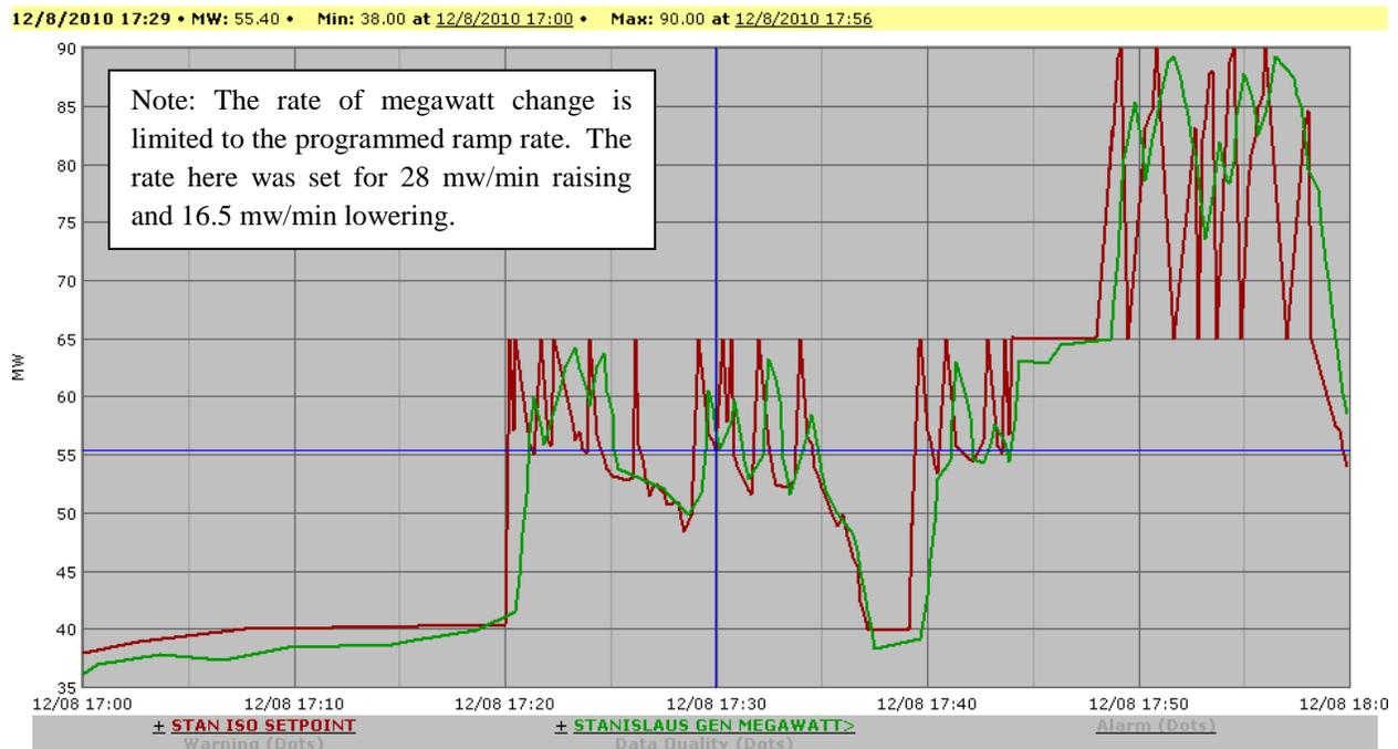
Figure 11 - Load Control at Stanislaus - Digital Governor - 1 Hour Window
