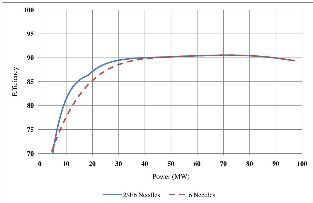
Figure 13 - Turbine Efficiency at Stanislaus - Needle Sequencing On vs. Off
