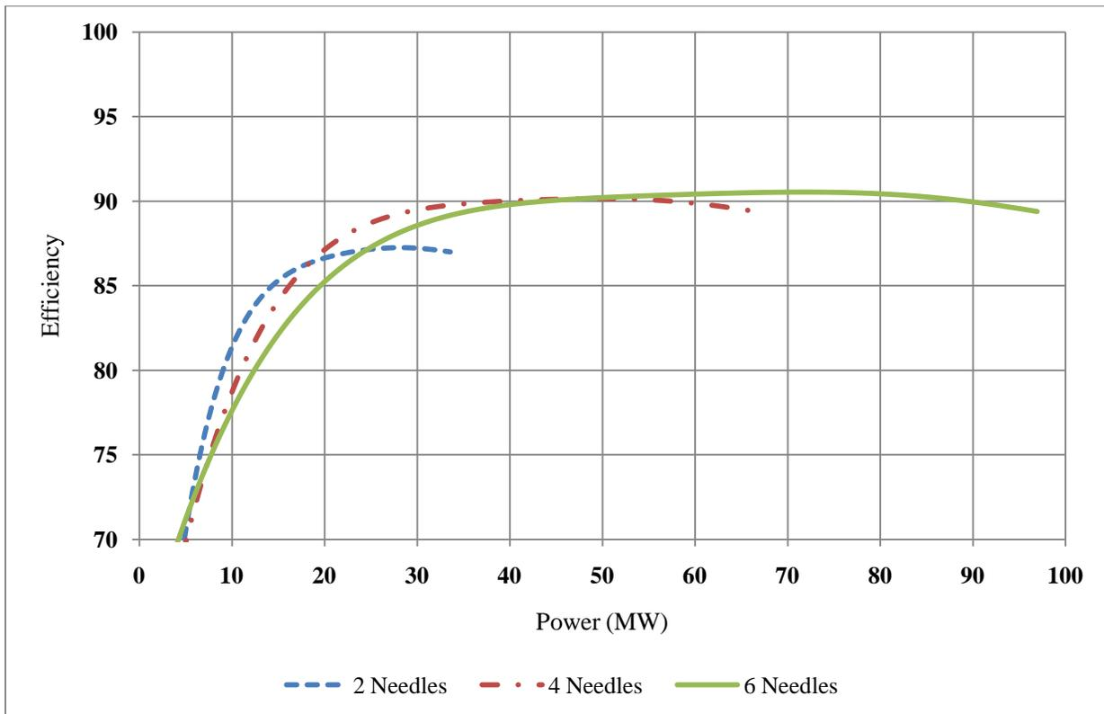
Figure 2 – Turbine Efficiency for 2, 4 and 6 Needle Operation at Stanislaus Powerhouse
