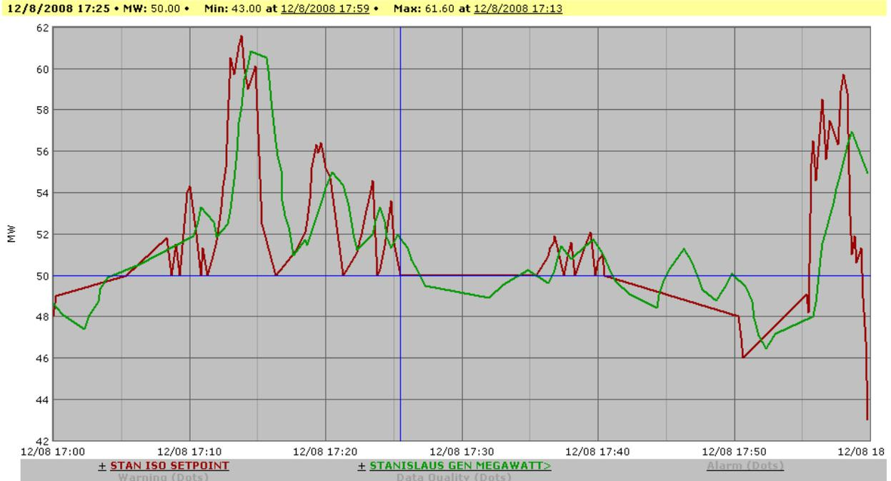
Figure 9 - Load Control at Stanislaus - Mechanical Governor - 1 Hour Window
