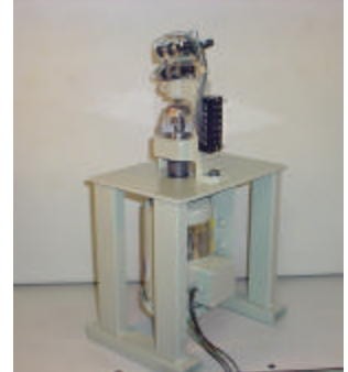
Auxiliary Speed Switch Under Test
