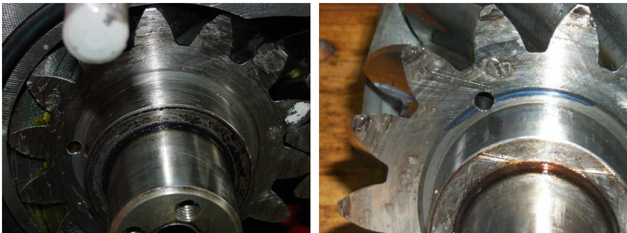
Figure 3 - Pump Gear Damage
